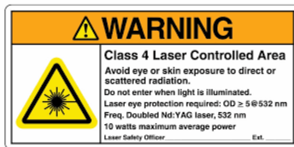
Figure 8b: Sample ANSI Z535.2 Compliant Warning Sign for Class 3B, Class 4 Lasers ( from ANSI Z136.1-2014 )
