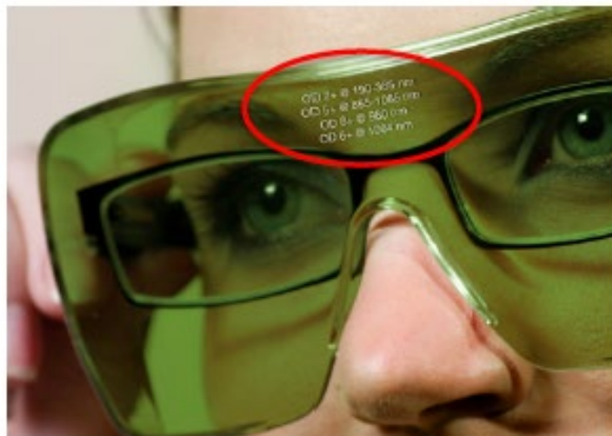
Figure 7: Legible ODs and wavelengths from the manufacturer must be visible and legible on the laser safety eyewear being used.
