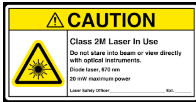
Figure 8a: Sample ANSI Z535.2 Compliant Caution Sign for Class 2, Class 2M and Class 3R Lasers ( from ANSI Z136.1-2014 )
