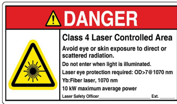
Figure 8c: Sample ANSI Z535.2 Compliant Class 4 Laser Controlled Area Danger Sign Format (from ANSI Z136.1-2014)
