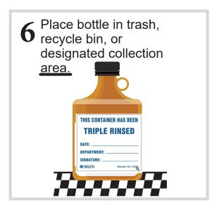
Do <u>not</u> triple rinse containers with sludge, solidified material, more than residual chemicals or septum caps. Submit as chemical waste instead.
