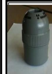
**Outer Source Containers (Pig)** must be kept separate from regular dry radioactive waste. In addition **ALL** source containers must be returned to Environmental Health & Safety for disposal.
